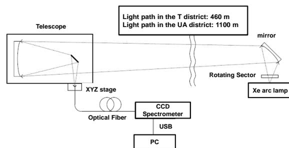
**Figure 2. Open-path DOAS instrumentation for the observation of  $\text{SO}_2$  concentration.**
