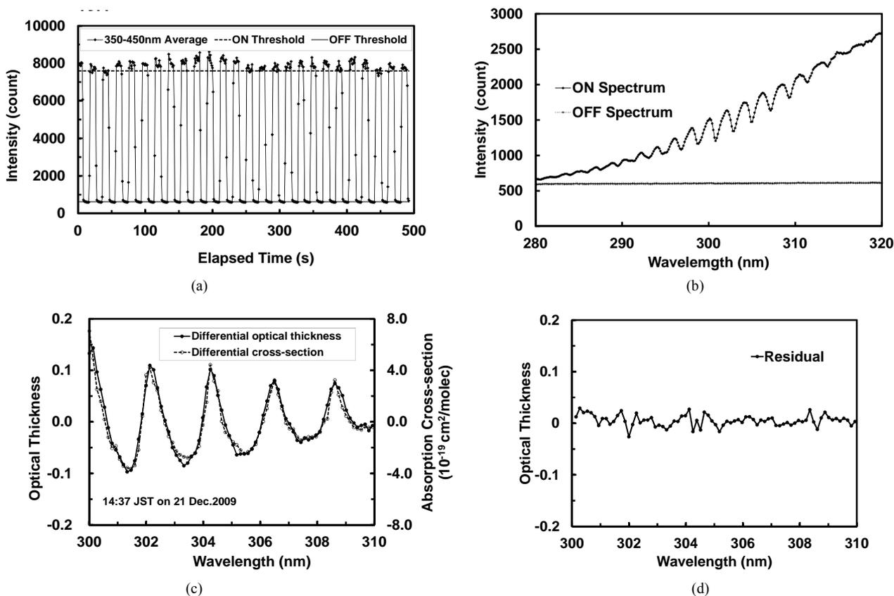
**Figure 4.** Analysis of observed DOAS spectra: (a) intensity variation observed during 500 s with a light path length of 460 m, (b) wavelength dependence of the resulting spectra for both off and on conditions, (c) comparison between the differential optical thickness ( $\Delta\tau$ ) of the DOAS spectrum and differential absorption cross-section ( $\Delta\sigma$ ) from reference Vandaele *et al.* (1994), and (d) the residual optical thickness after the fitting procedure.
