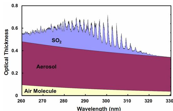
**Figure 3. Wavelength dependence of each optical thickness component simulated for the wavelength range of 260 nm - 330 nm. It is noted that  $\text{SO}_2$  absorption exhibits notable spectral features, whereas aerosol and air-molecule extinction show less prominent wavelength dependence.**
