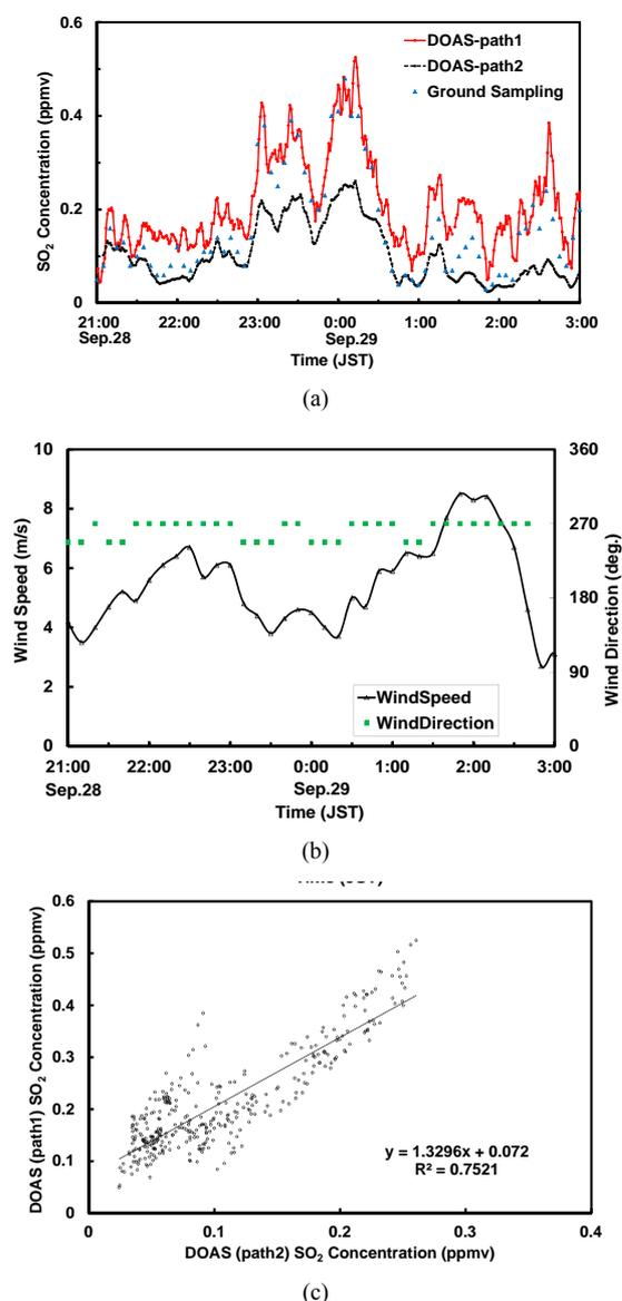
**Figure 9.** Result of the double-path DOAS observation conducted in the T district during 28-29 September 2010: (a) SO<sub>2</sub> concentration from the double-path DOAS and sampling measurements, (b) wind speed and wind direction, and (c) correlation between the two DOAS paths: one data point indicates the 5 min average for both paths.
