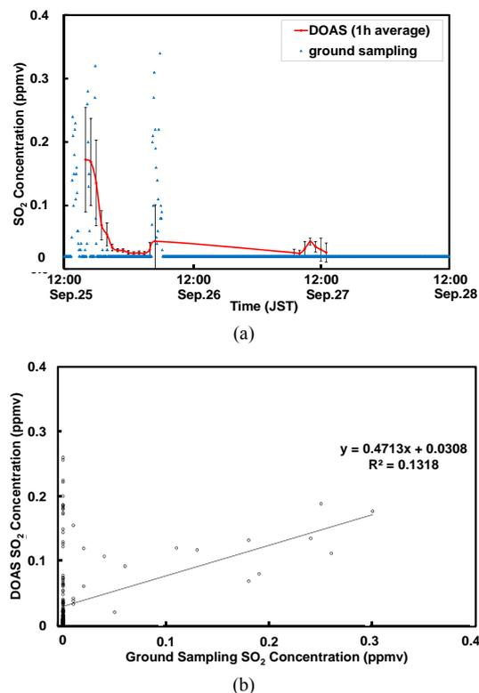
**Figure 8.** Temporal variation of SO<sub>2</sub> concentration from DOAS and ground sampling measurements in the UA district during 25-28 September 2010, and (b) correlation between the results of the DOAS (5 min average) and ground sampling measurements (230 data points).
