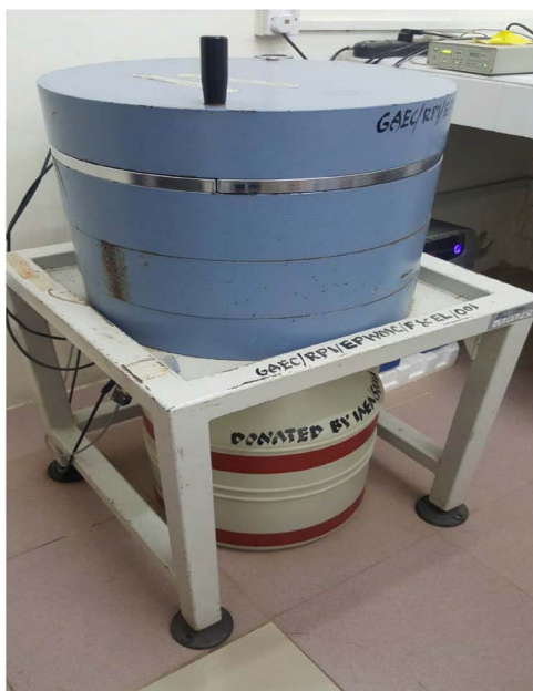
Figure 7. Shows a lead shield which is the blue equipment on top is used to cut off the background radiation from interfering with the actual concentration of the radionuclides been measured. While the equipment below which is known as Dewar contain liquid nitrogen for cooling the High Pure Germanium Detector during analysis of the borehole water samples.
