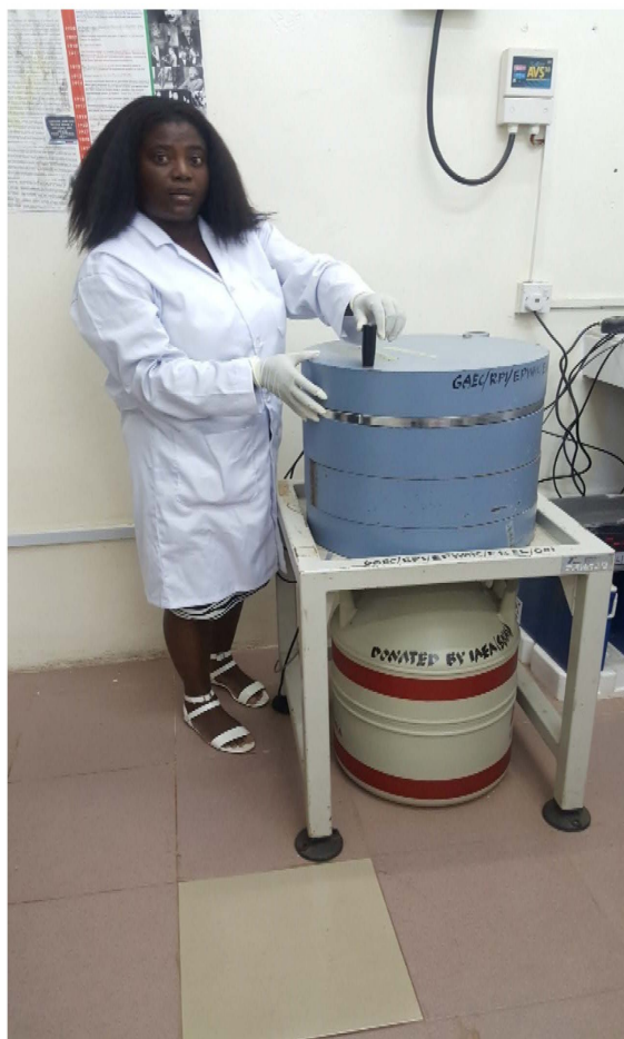
Figure 6. Shows norms measurement been carried out by a laboratory technologist using the high pure germanium detector (HPGe Detector).
