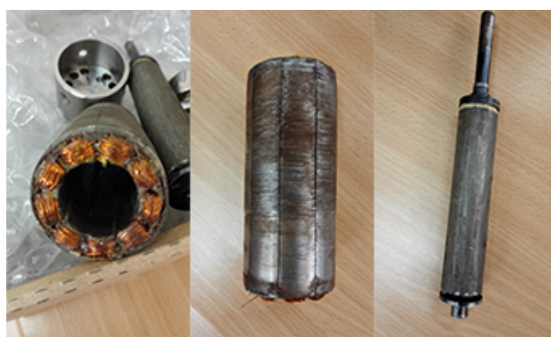
Figure 6. Structure diagram of rotor and stator.
