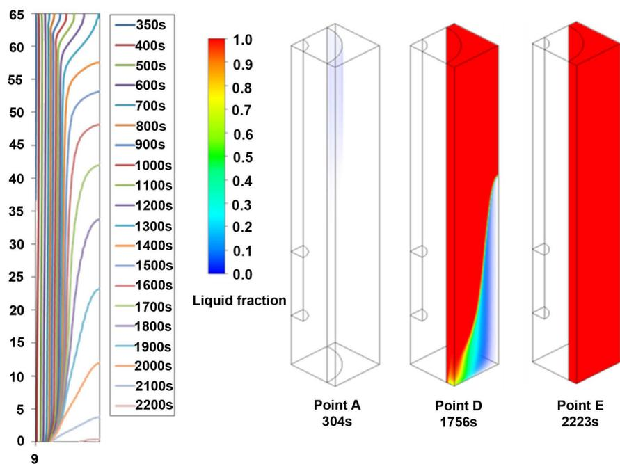
**Figure 6.** The solid-liquid interface of the PCM at the A-A cross section during the melting process and the visualization of the PCM liquid fraction behind B-B cross section.
