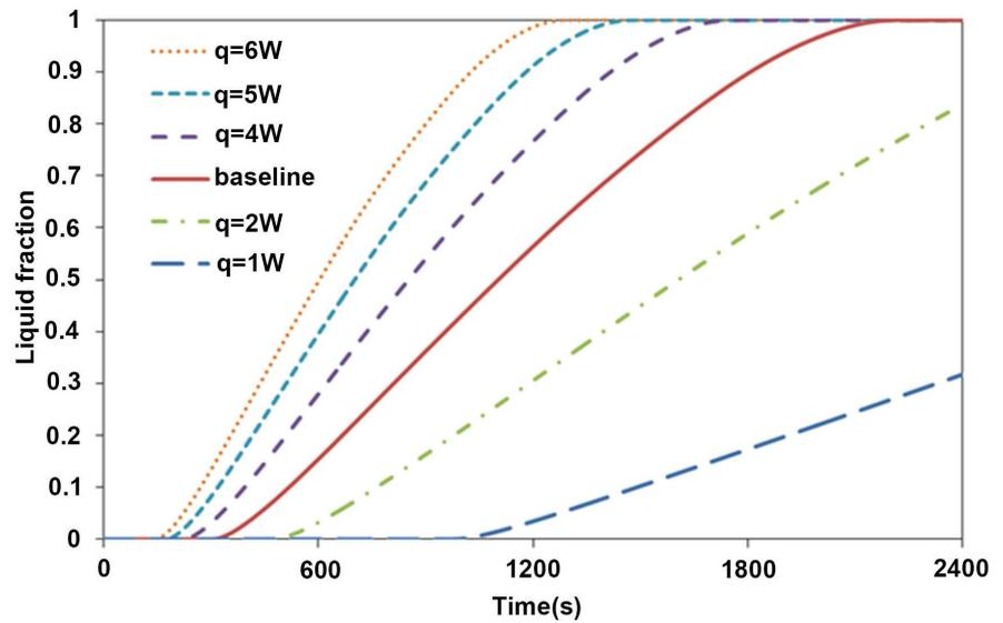
**Figure 5.** The PCM liquid fraction evolutions under the PCM passive thermal management at different heating powers.
