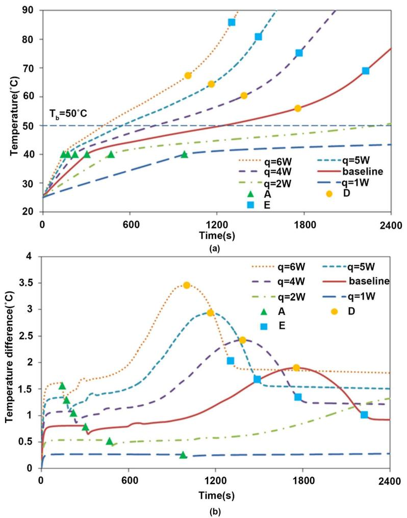
**Figure 4.** The battery temperature results under the PCM passive thermal management at different heating powers. (a) Battery temperature evolutions; (b) the temperature difference between battery top and bottom.
