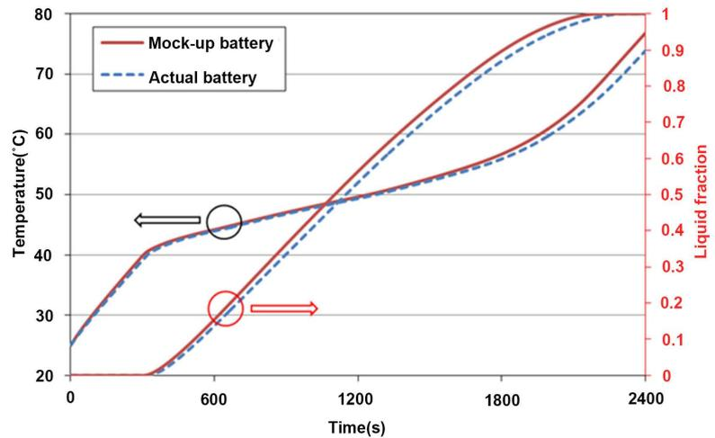
**Figure 3.** The comparisons of the battery temperature rise and the PCM liquid fraction between the mock-up and the real batteries.
