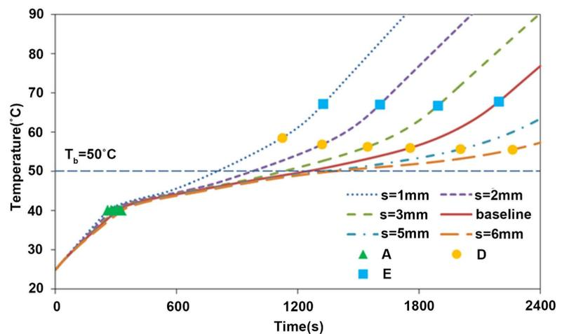
**Figure 8.** The battery temperature evolutions under different battery spacings at the heating power of 3 W.
