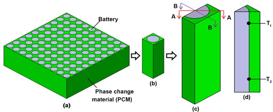
**Figure 1.** Numerical model of the PCM thermal management system, (a) the overall system, (b) the single battery numerical model, (c) the 1/2 battery numerical model, (d) the schematic of the temperature monitoring points in A-A cross section.
