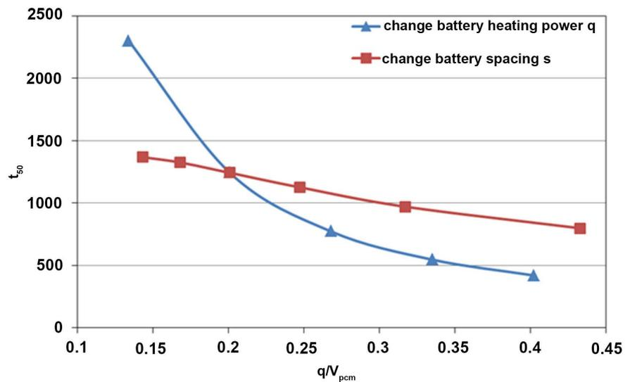
**Figure 9.** The results of the  $t_{50}$  at different  $q/V_{pcm}$  while varying the battery heating power or the battery spacings.
