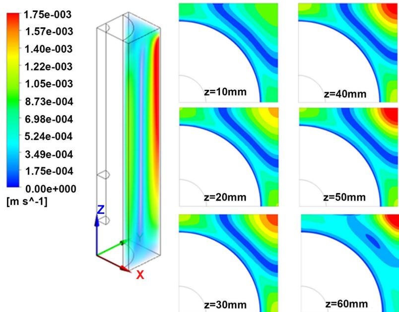
**Figure 7.** The velocity distribution of the liquid PCM and the velocity contours at different heights of the battery at the characteristic point of E.
