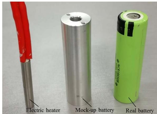
**Figure 2.** The mock-up and the real cylindrical batteries.
