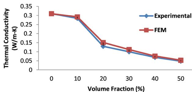
**Figure 6.** Thermal conductivity of epoxy composites as a function of filler content.
