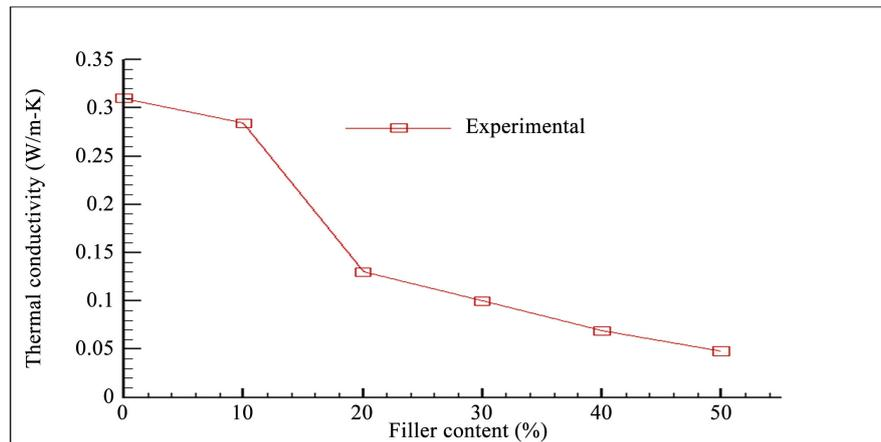
**Figure 3.** Thermal conductivity of epoxy composites as a function of filler content (Rice husk).
