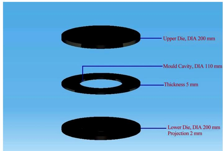
**Figure 1.** Mould to cast specimens for Lee's Apparatus.
