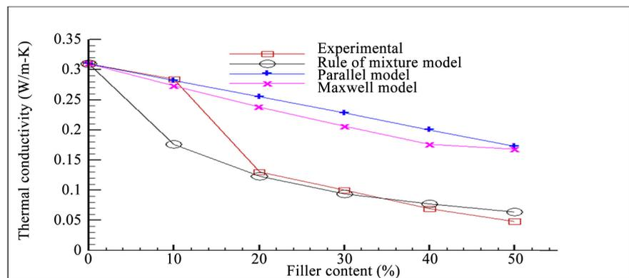
**Figure 4.** Comparison of thermal conductivity values obtained from different model.
