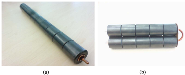
Figure 7. Coaxial transformer prototype built for one (a) and two tubes (b).
