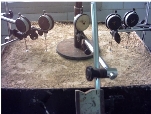
**Figure 4.** Plat loading test at 25 cm base thickness.
