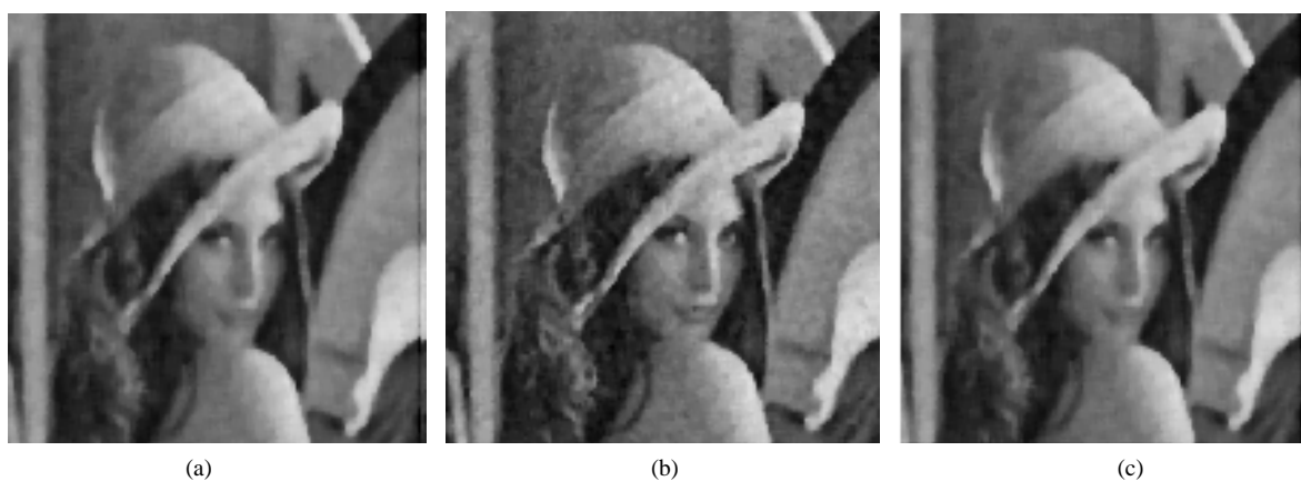
Figure 4. Results of median filtering. (a) 3 \times 3 template; (b) 5 \times 5 template; (c) 7 \times 7 template.
