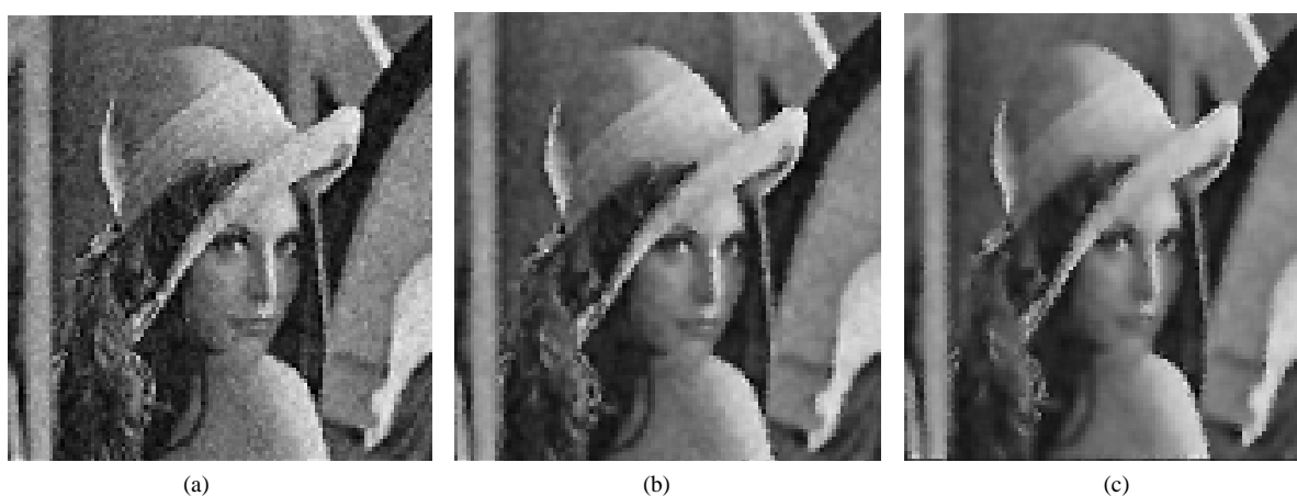
Figure 5. Results of wiener filtering. (a) 3 \times 3 template; (b) 5 \times 5 template; (c) 7 \times 7 template.
