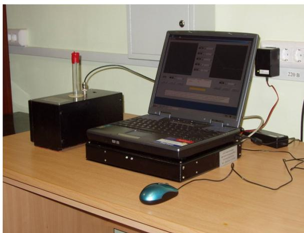
**Figure 1.** Portable low field NMR-relaxometer.
