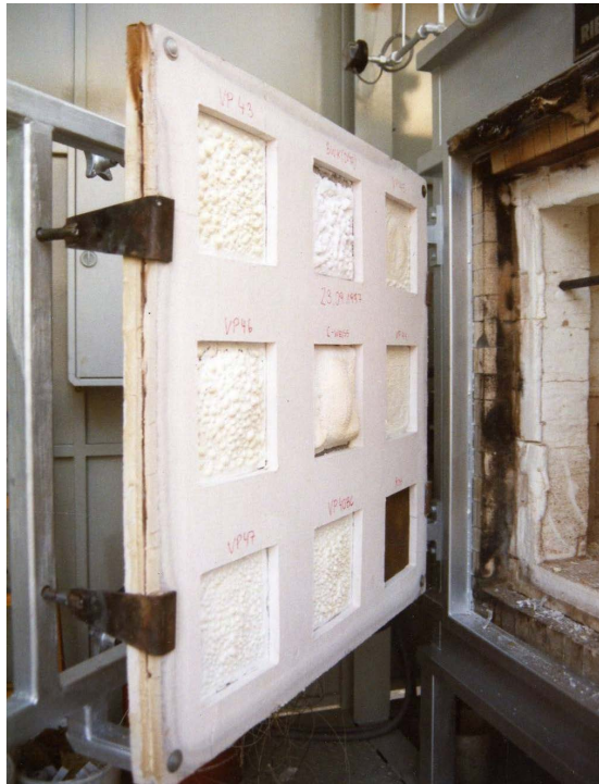
Figure 9. The front side after the burning test showing the 7 samples No. 1, No. 2, No. 3, No. 4, No. 5, No. 6, No. 7, the uncoated panel and the reference panel Nonfire S168.
