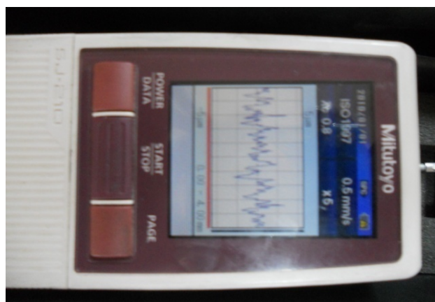
Figure 3. Mitutoyo Surface Roughness tester SJ 210.
