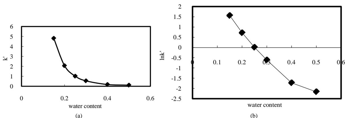
**Figure 2.** (a) Plot of retention factor ( $k'$ ) versus the content of water in the mobile phase. (b) Plot of  $\ln k'$  versus the content of water in the mobile phase. Column temperature: 35°C. Flow rate: 1.5 mL/min. Sample: HP- $\beta$ -CD (3.0 mg/mL) dissolved in the mobile phase. Injection volume: 20  $\mu$ L.
