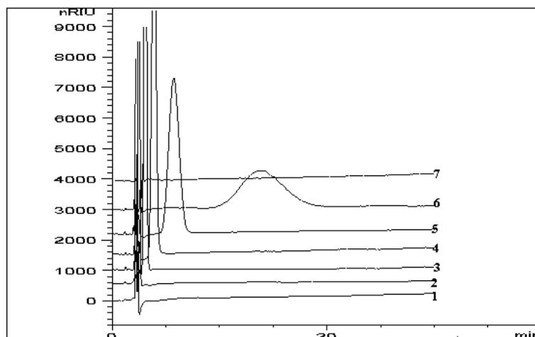
**Figure 1.** Chromatograms of different water contents in the mobile phase: (1) 50% water, (2) 40% water, (3) 30% water, (4) 25% water, (5) 20% water, (6) 15% water, (7) 10% water. Column temperature: 35°C. Flow rate: 1.5 mL/min. Sample: HP- $\beta$ -CD (3.0 mg/mL) dissolved in the mobile phase. Injection volume: 20  $\mu$ L.
