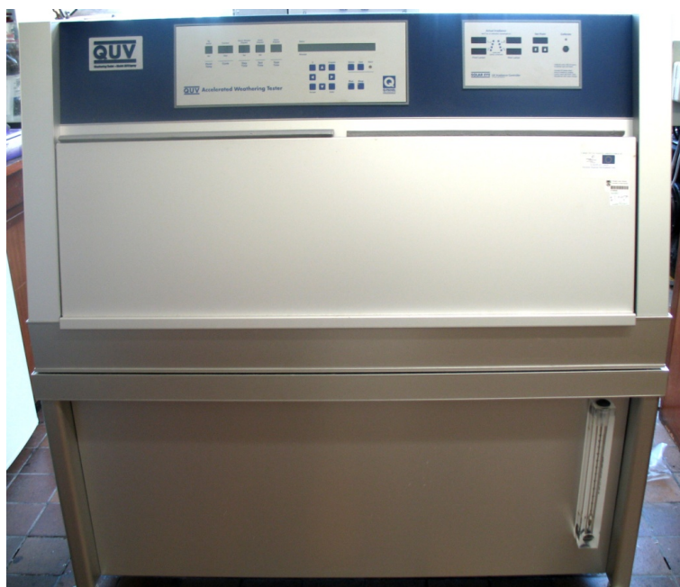
Figure 2. QUV accelerated weathering testing machine.
