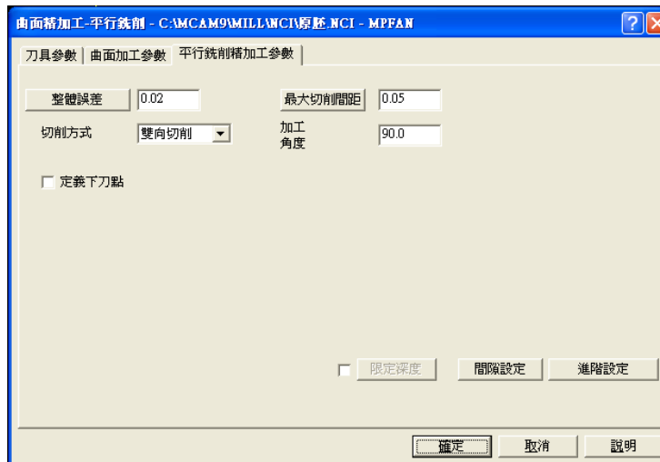
Figure 2. Tool parameter settings of surface finish.
