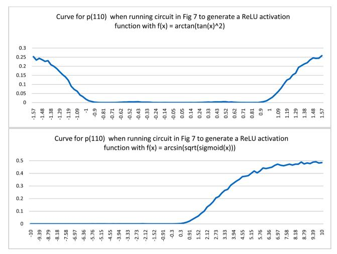
Figure 8. ReLU functions generated by the activation function in [9] (top plot) and ours (bottom plot) using the circuit in Figure 8. P(110) means the probability of seeing 110 in the three measure-
