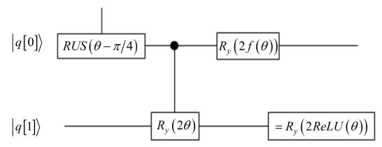
Figure 7. A circuit created in [9] to use their nonlinear activation function to generate the ReLU function (Figure 9 in [9]).
