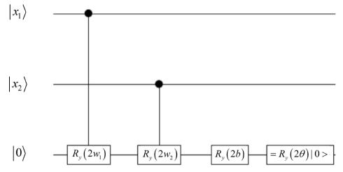
Figure 4. A circuit created in [9] to train the quantum neurons (Figure 4(c) in [9]) using equation  $\theta = w_1 * x_1 + w_2 * x_2 + b$ .
