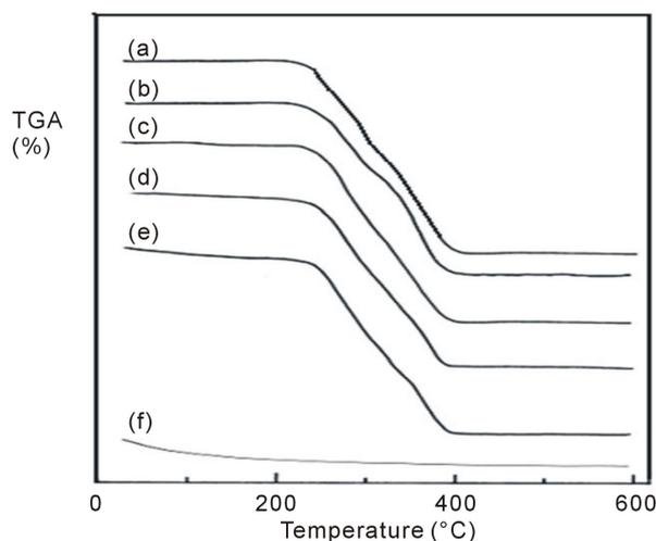
**Figure 1.** TGA curves of PMMA/TiO<sub>2</sub> nanoparticles composites: (a) 100/0, (b) 97.5/2.5, (c) 95/5, (d) 92.5/7.5, (e) 90/10 and (f) 0/100 (wt/wt%).
