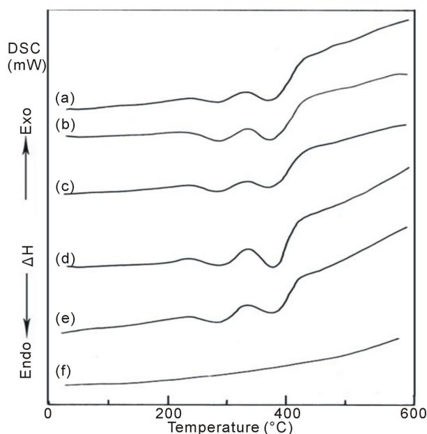
**Figure 3.** DSC curves of PMMA/TiO<sub>2</sub> nanoparticles composites: (a) 100/0, (b) 97.5/2.5, (c) 95/5, (d) 92.5/7.5, (e) 90/10 and (f) 0/100 (wt/wt%).
