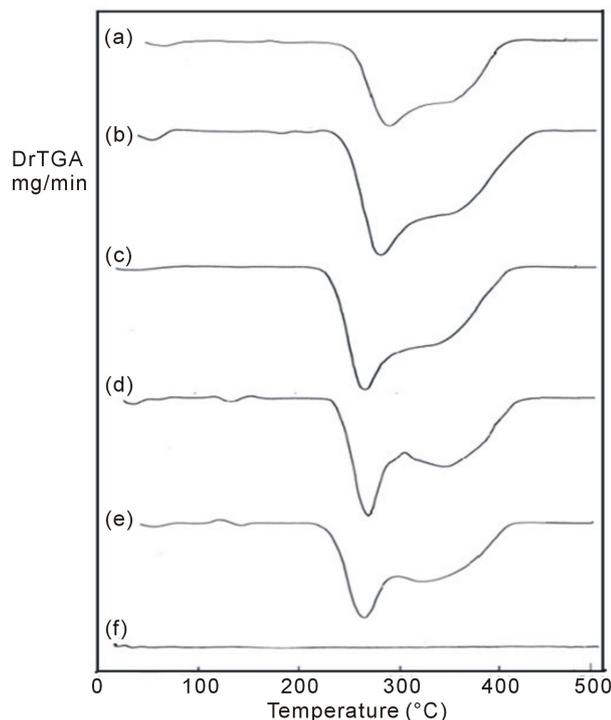
**Figure 2.** DrTGA curves of PMMA/TiO<sub>2</sub> nanoparticles composites: (a) 100/0, (b) 97.5/2.5, (c) 95/5, (d) 92.5/7.5, (e) 90/10 and (f) 0/100 (wt/wt%).
