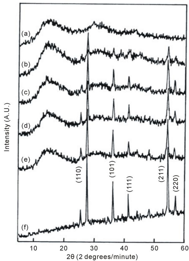
**Figure 4.** Variation in X-ray diffraction patterns of PMMA/TiO<sub>2</sub> nanoparticles composites: (a) 100/0, (b) 97.5/2.5, (c) 95/5, (d) 92.5/7.5, (e) 90/10 and (f) 0/100 (wt/wt%).
