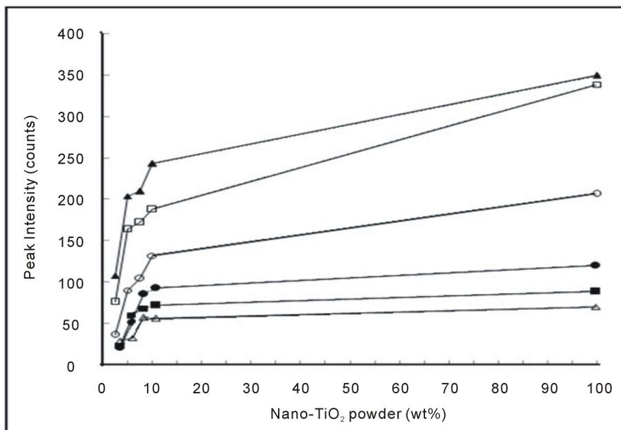
**Figure 5.** Variation of peaks intensity of XRD patterns at different angles for PMMA/TiO<sub>2</sub> nanoparticles composites: at  $2\theta$ : ( $\Delta$ ) 25.27 - 25.43, ( $\blacktriangle$ ) 27.39 - 27.56, (o) 36.01 - 36.22, ( $\bullet$ ) 41.16 - 41.34, ( $\square$ ) 54.23 - 54.43 and ( $\blacksquare$ ) 56.58 - 56.78 degrees.
