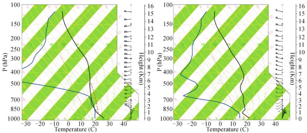
**Figure 8.** Skew-T plots of Lihue soundings valid at 0000 UTC 30 (left) and 31 (right) January 2010, based on the experiment without GPS RO assimilation. The black (blue) thick line represents the temperature (dew point temperature) profile.
