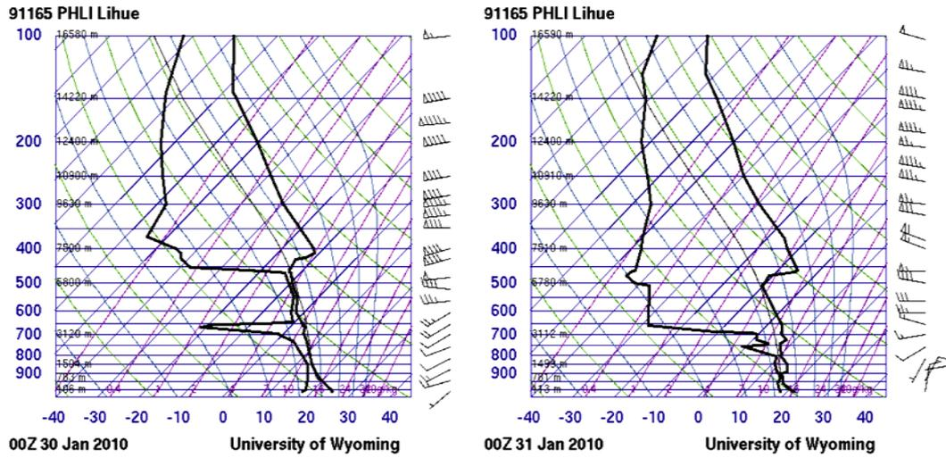
**Figure 7.** Skew-T plots of Lihue soundings at 0000 UTC 30 (left) and 31 (right) January 2010. The black thick line on the left (right) of each panel represents the profile of temperature (dew point temperature). These figures were downloaded from the University of Wyoming (<http://weather.uwyo.edu/upperair/sounding.html>).
