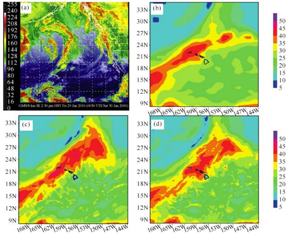
**Figure 5.** (a) Satellite image at 0030 UTC 30 January, 2010; (b) Total precipitable water at 0000 UTC 30 January, 2010 from NCEP FNL; (c) Total precipitable water at 0000 UTC 30 January, 2010 from the GPS RO run; (d) Total precipitable water at 0000 UTC 30 January, 2010 from the no-GPS RO run.
