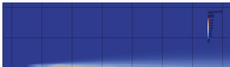
Figure 3. Time average of the vertical cross section of \text{NO}_x concentration spatial distribution (in \mu\text{g}\cdot\text{m}^{-3} ) in the case of none barrier.
