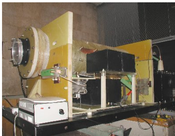
Figure 1. TC-300. Electrical discharge CO 2 laser with output—300 J.
