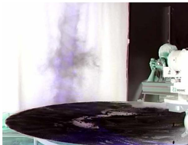
**Figure 6.** A typical frame (negative) with a registered vortex (mode No. 6); magnesia particles visualization, the image size is 1.0 by 0.75 m.
