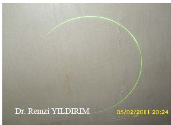
Figure 9. The green laser light bending as a part of a circle with one-piece lens.
