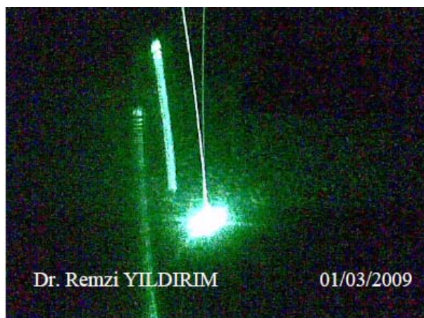
Figure 11. The single green laser light that is obtained from the laser source separation and different deflected in four parts.
