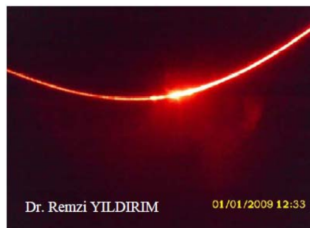
Figure 6. One-piece lens with the red laser light bending in a parabola.
