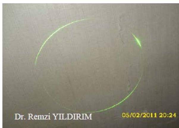
Figure 10. The green laser light bending as parts of a circle with one-piece lens.
