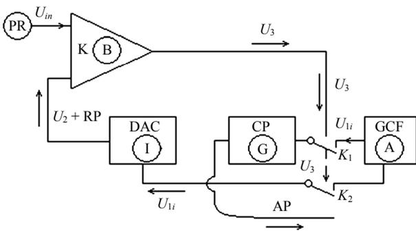
**Figure 3.** Equivalent circuit of a neural network retina:  $K_1, K_2$ —keys.
