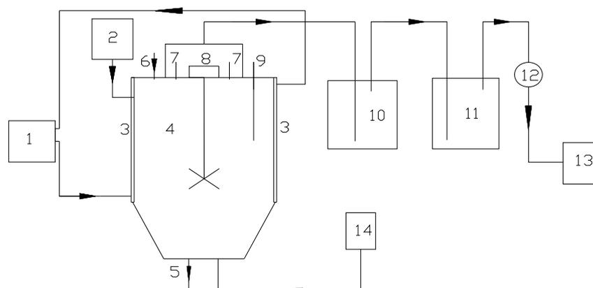
1. SC-15 water bath; 2. pH adjusting port; 3. organic reactor; 4. agitating blade; 5. reaction substrate outlet; 6. material inlet; 7. vent; 8. digital stirrer; 9. thermometer; 10. CO<sub>2</sub> removal; 11. desiccant; 12. wet gas flowmeter; 13. GC-7900 gas chromatography; 14. nitrogen purging port.
