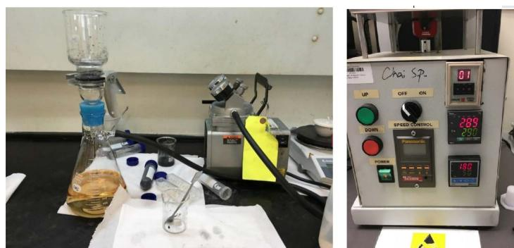
**Figure 2.** Synthesis rGO-TiO<sub>2</sub> (S) via solvothermal method by using a Teflon-Lined autoclave.
