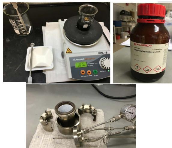
**Figure 3.** Synthesis rGO-TiO<sub>2</sub> (H1) and rGO-TiO<sub>2</sub> (H2) via hydrothermal method by using a Teflon-Lined autoclave.
