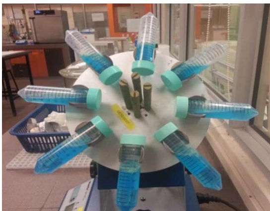
Figure 3. Rotator (Digital Feedback Controlled Rotator) with tested samples of SGB and MB.
