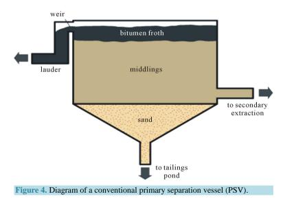
the PSV. Material of intermediate density, called middlings, are collected into a third stream and sent to flotation cells for further bitumen recovery. In these flotation cells, air is delivered to the machine establishing bubble dispersions for bitumen-air attachment, allowing bitumen froth to be recovered at the top of the flotation machines while the remaining pulp exits through the bottom of the machines. The recovered bitumen froth is re-circulated to the PSV for further processing.
