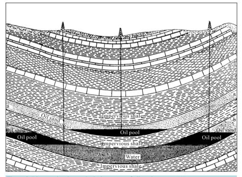
Figure 2. Diagram showing geological structure of oil sands reserves [1].
