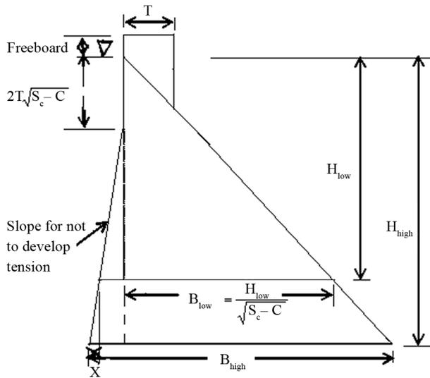
Figure 1. Typical section of a high concrete gravity dam.
