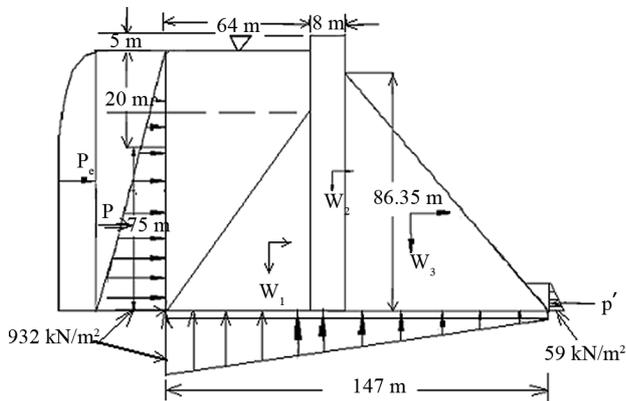
Figure 2. High concrete gravity dam with external forces.
