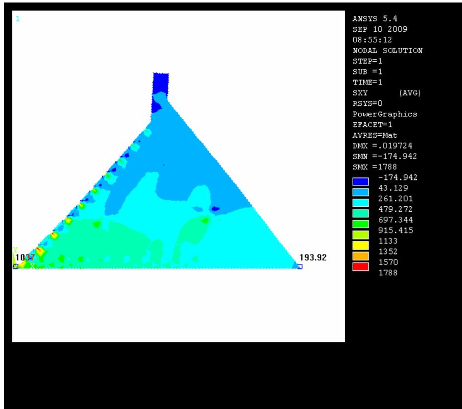
Figure 3. Contour plot of shear stress ( $\tau$ ).
