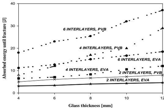
**Figure 7. Absorbed energy until fracture by Charpy impact test when the inner thickness is variable and the bonding material is PVB and EVA.**
