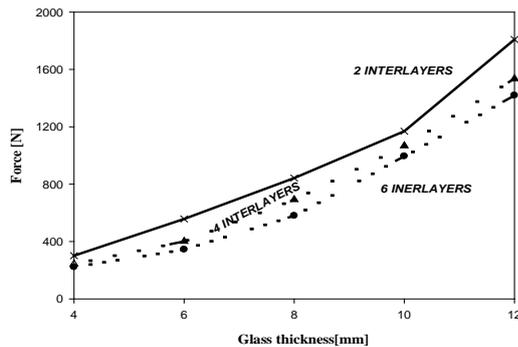
Figure 3. Testing the maximum force on (PVB) laminated glass where the thickness of outer plate was fixed and the inner plate was fixed and the inner plate and interlayer were changeable.
