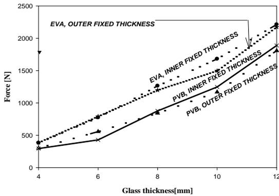
**Figure 6. Comparison of the maximum load capacity for the 2 or fixed interlayer thickness, variable bonding material, and different positions of glass thicknesses.**
