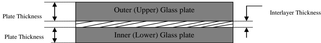
Figure 1. Schematic diagram for the assembly of the glass plates and interlayer. Outer glass is the one in contact with the applied force.
