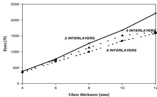
Figure 4. Testing the maximum force on (EVA) laminated glass where the thickness of inner plate was fixed and the
