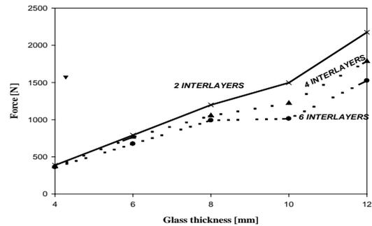
Figure 5. Testing the maximum force on (EVA) laminated glass where the thickness of outer plate was fixed and the outer plate and interlayer were changeable.
