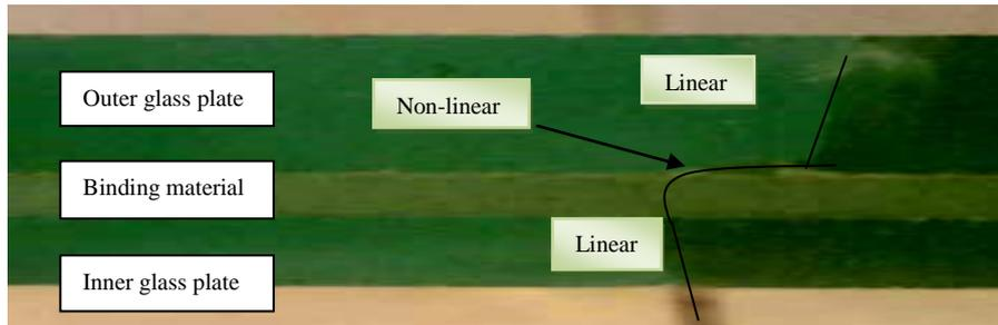
Figure 10. Failure observed after bending test (side view).
