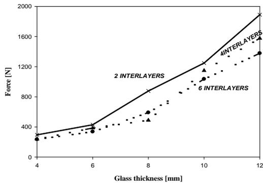
Figure 2. Testing the maximum force on (PVB) laminated glass where the thickness of inner plate was fixed and the outer plate was fixed and the outer plate and interlayer were changeable.
