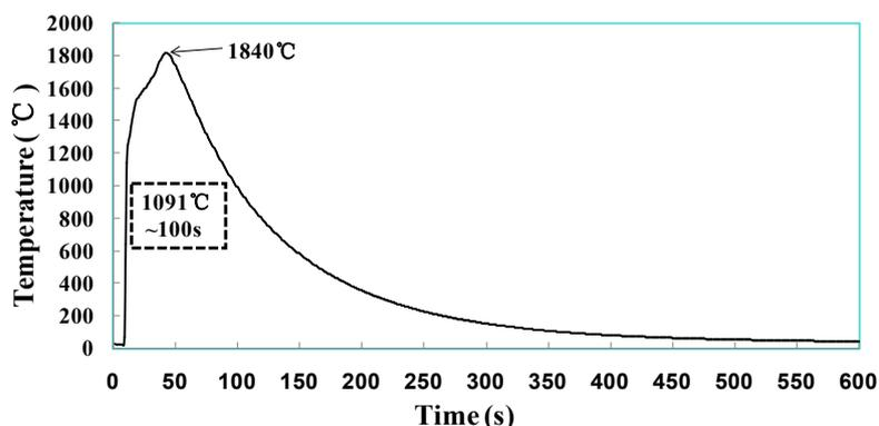
**Figure 2.** Temperature history of sample M-2 at CS under 0.7 MPa  $N_2$  pressure, the thermal couples were set at the center of the sample.
