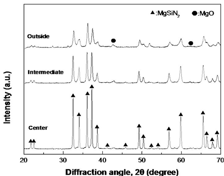
Figure 5. XRD patterns of the combustion product of sample M-2.
