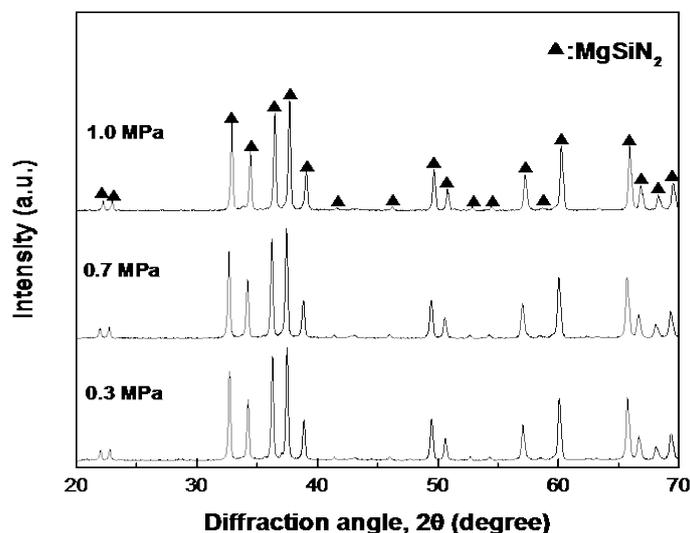
Figure 4. XRD patterns of combustion product synthesized at different  $N_2$  pressures.
