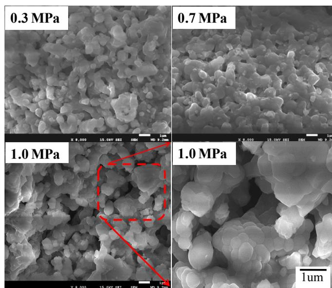
**Figure 6.** SEM images of combustion products synthesized at different  $\text{N}_2$  pressures.
