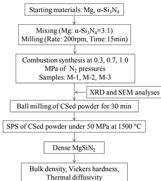
**Figure 1.** Flow chart of the experimental procedure for synthesizing MgSiN<sub>2</sub>.
