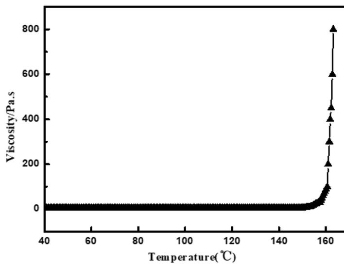
**Figure 3.** Viscosity vs temperature for BSA resin.
