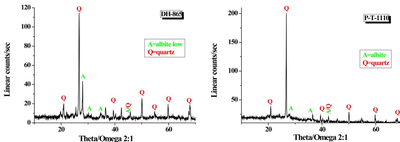
**Figure 6.** XRD spectra of two representative samples.
