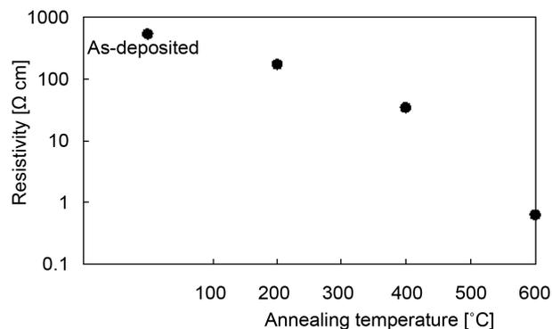
**Figure 4.** The resistivity of the deposited film as a function of the annealing temperature. It is noticeably decreases with the annealing temperature even over 400°C.
