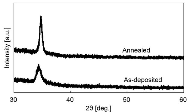
**Figure 1.** X-ray diffraction spectra from the samples that were as-deposited (lower) and annealed at 600°C (upper). Only one reflection peak assigned to (002) diffraction was observed in the both spectra.
