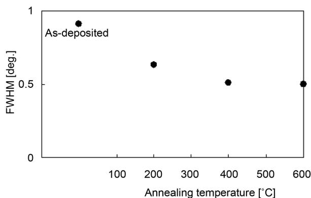
**Figure 3.** The FWHM of the (002) peak as a function of the annealing temperature. At 400°C, the FWHM is lowered enough.
