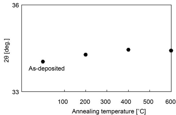
**Figure 2.** The dependence of the (002) peak position on the annealing temperature. The peak shift from 34.47 degree was completely vanished over 400°C.
