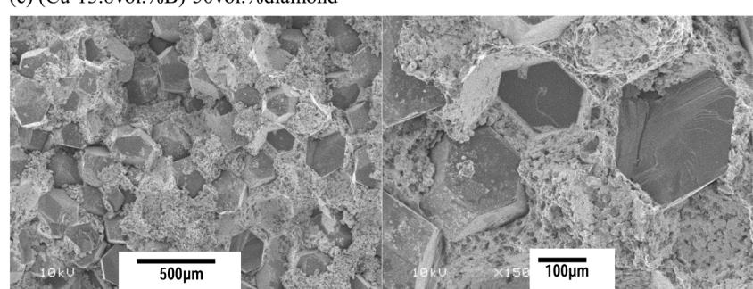
**Figure 11.** Bending fracture surfaces of diamond particle dispersed Cu matrix composites fabricated by spark plasma sintering (left: low magnification, right: high magnification). (a) Cu-50vol.% diamond composite, (b) (Cu-7.2 vol.%B)-50vol.% diamond composite and (c) (Cu-13.8 vol.%B) -50vol.% diamond composite.
