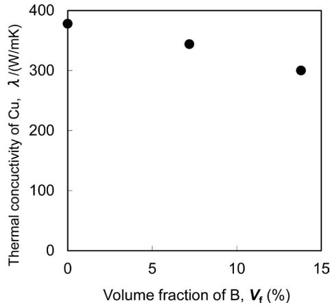
**Figure 7.** Change in the thermal conductivity of Cu consolidated by spark plasma sintering (SPS) as a function of the boron content.
