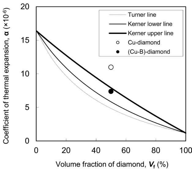
**Figure 12.** Comparison of coefficients of the thermal expansion predicted theoretically using Kerner model for Cu and Diamond composite and those obtained experimentally for Cu-50 vol. % diamond and (Cu-7.2 vol.%B)-50 vol.% diamond composite. Turner line obtained theoretically is also depicted.
