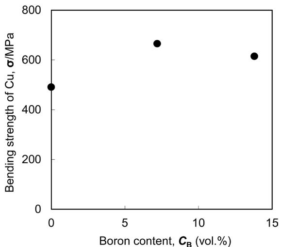
**Figure 9.** Change in the bending strength of Cu consolidated by spark plasma sintering (SPS) as a function of the boron content in Cu.
