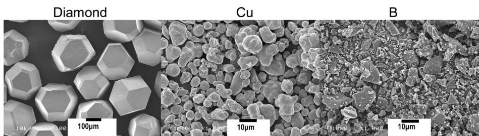
**Figure 1.** SEM micrographs of as-received diamond, Cu and B powders, showing the powder morphology.
