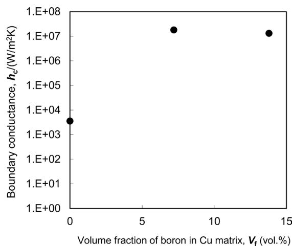
**Figure 8.** Change in the boundary conductance of (Cu-B)-50vol.% diamond composites as a function of the boron content in Cu matrix.
