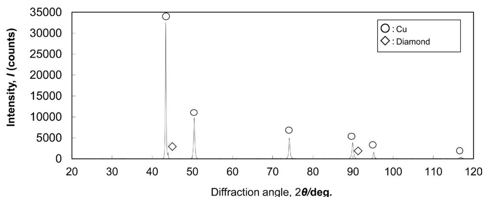
**Figure 5.** X-ray diffraction pattern taken from (Cu-7.2vol.%B)-50vol.%diamond composite fabricated by spark plasma sintering (SPS), showing two phases.
