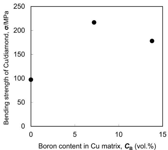
**Figure 10.** Change in the bending strength of (Cu-B)-50vol.% diamond composites fabricated by spark plasma sintering (SPS) as a function of the boron content in Cu matrix.
