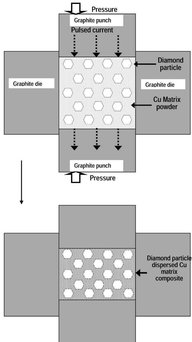
**Figure 2.** Schematic illustration showing processing of diamond particle dispersed Cu-matrix composite by spark plasma sintering (SPS).
