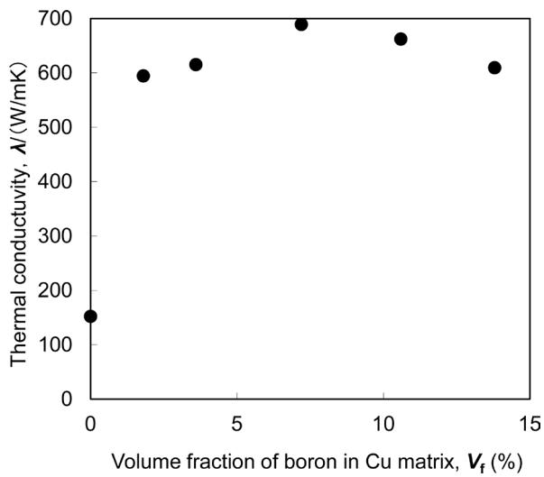
**Figure 6.** Change in the thermal conductivity of (Cu-B)-50vol.% diamond composites fabricated by spark plasma sintering (SPS) as a function of the boron content in Cu matrix.
