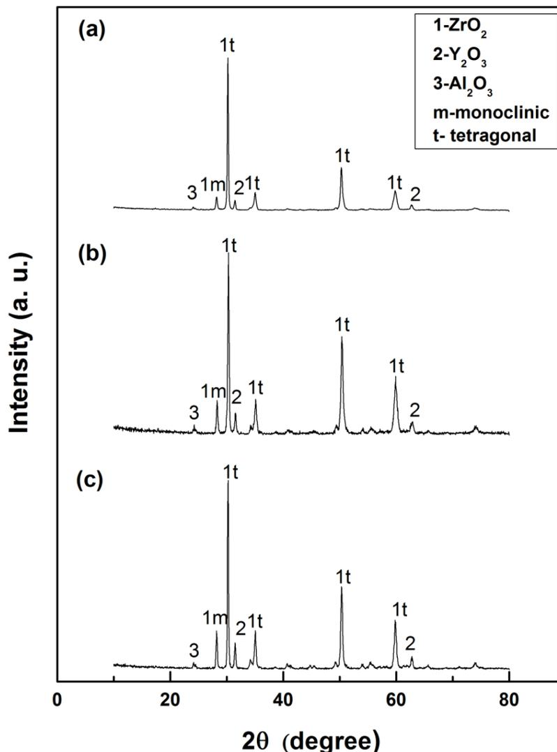
**Figure 3.** XRD analysis of (a) conventional, (b) microwave and (c) vacuum sintered  $0.5\text{Al}_2\text{O}_3\text{-YSZ}$  specimens.
