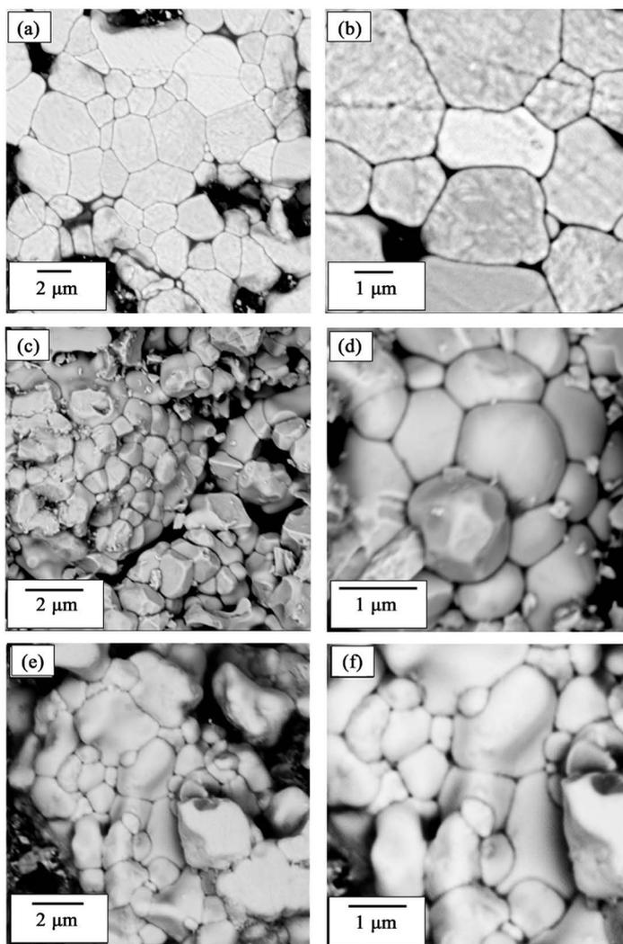
**Figure 4.** SEM images of (a)-(b) conventional, (c)-(d) microwave and (e)-(f) vacuum sintered 0.5 Al<sub>2</sub>O<sub>3</sub>-YSZ specimens.
