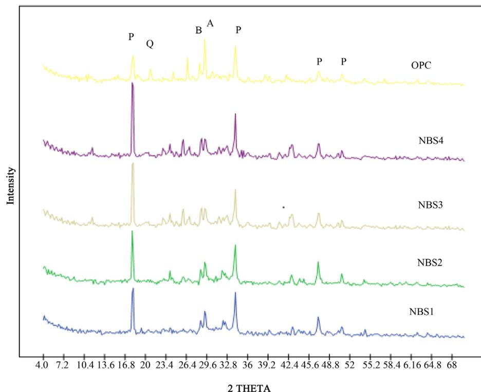
Figure 1. XRD patterns of samples hydrated up to 90 days (P = Portlandite, A = alite, B = Barite, Q = Quartz).
