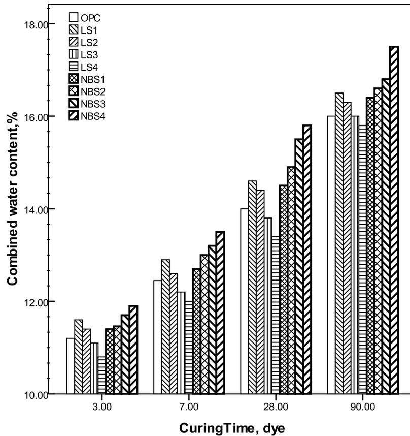
**Figure 2.** Chemically combined water content of the investigated mixes as a function of curing time.
