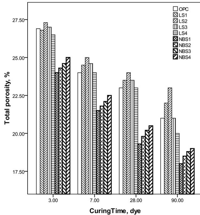
Figure 4. Total porosity of the investigated mixes as a function of curing time.
