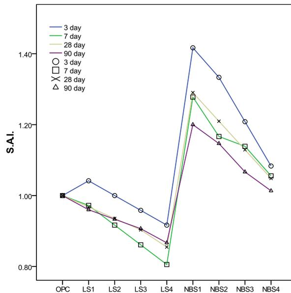
Figure 6. The strength activity index values for each age against the filler materials.
