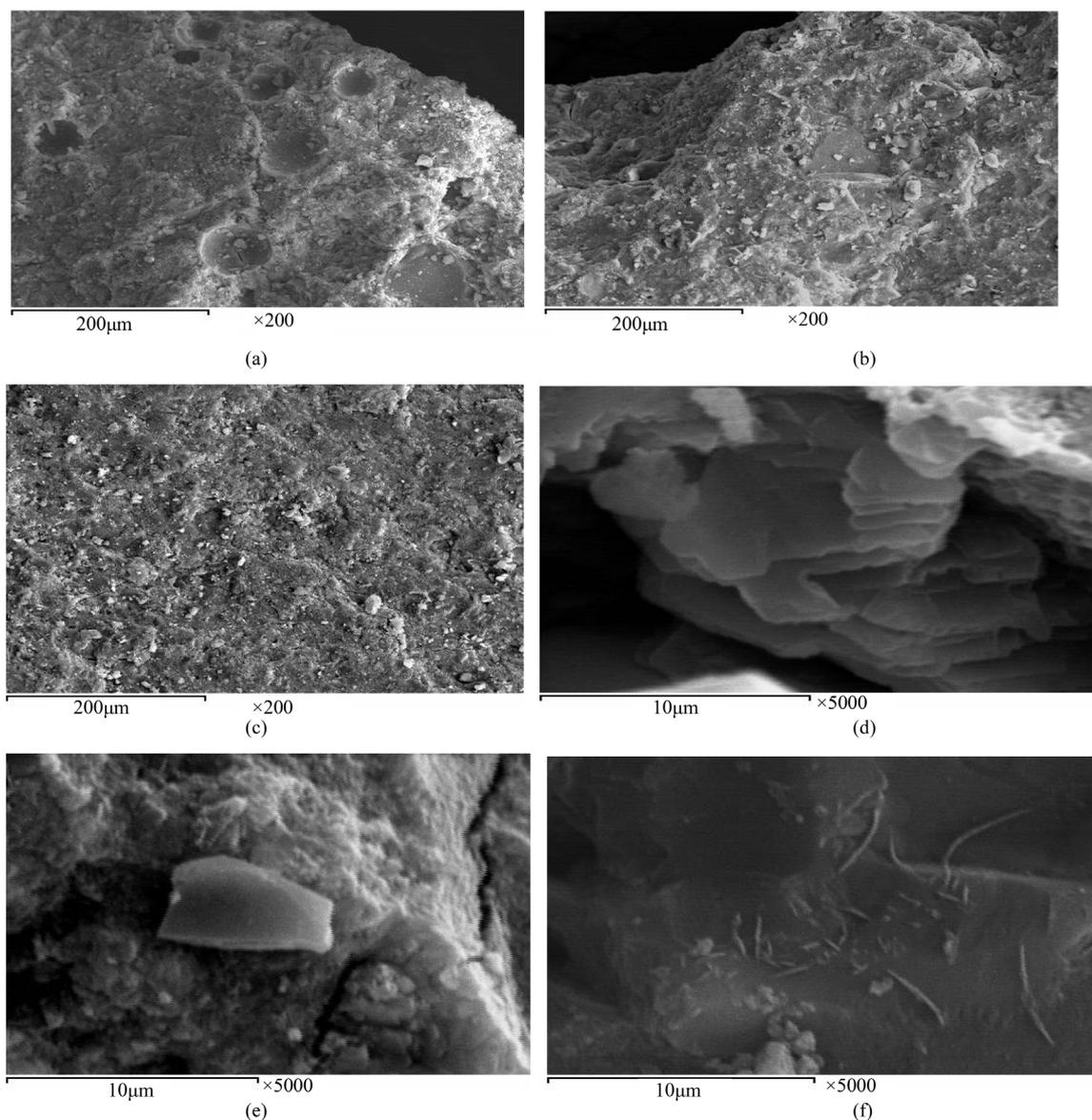
**Figure 7.** SEM micrographs of OPC, NBS1, and NBS2 Mixes hydrated up to 90 days.
