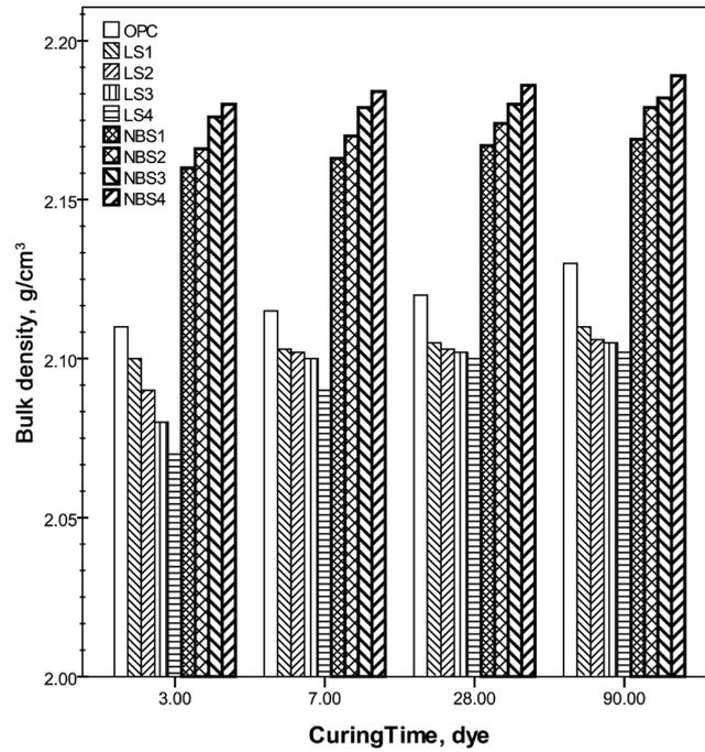
Figure 3. Bulk density of the investigated mixes as a function of curing time.
