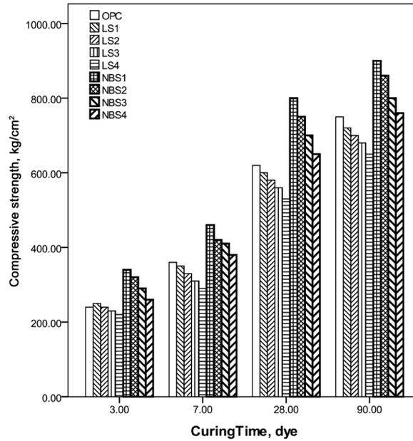
Figure 5. Compressive strength of the investigated batches as a function of curing time.
