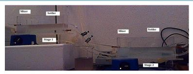
Figure 1. Laboratory mixer-settler (2 stages).
