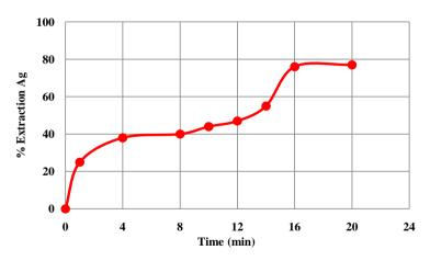
**Figure 3.** Effect of the extraction time on the Ag extraction. Phase ratio A/O =  $1, 22^{\circ}C \pm 1^{\circ}C$ .
