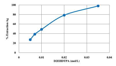
**Figure 2.** Effect of the extractant concentration on the Ag extraction. Phase ratio  $A/O = 1, 22^{\circ}C \pm 1^{\circ}C$ .
