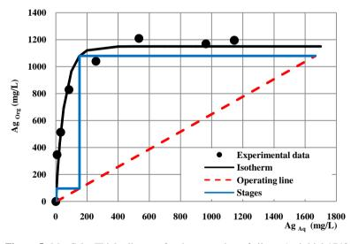
**Figure 5.** MacCabe-Thiele diagram for the extraction of silver, Ag initial 1743 mg/L. Organic phase: D2EHDTPA 0.02 mol/L time 15 minutes and  $22^{\circ}C \pm 1^{\circ}C$  A/O = 0.65.
