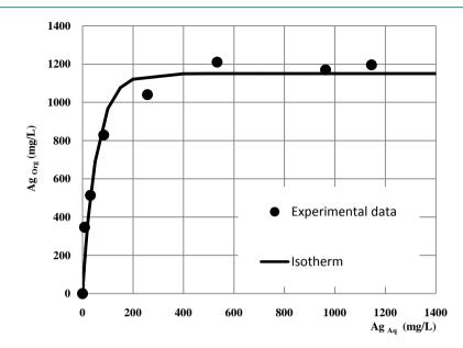
**Figure 4.** Isoterm of silver extraction. Aqueous phase: Ag initial 1803 mg/L. Organic phase: D2EHDTPA 0.02 mol/L time 15 minutes and  $22^{\circ}C \pm 1^{\circ}C$ .
