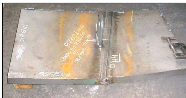
Figure 7. The body-of-proof (BP) used in the experiments (qualification).
