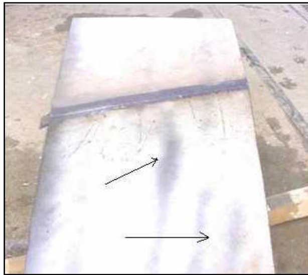
Figure 10. The BP presented dark spots after heat treatment.
