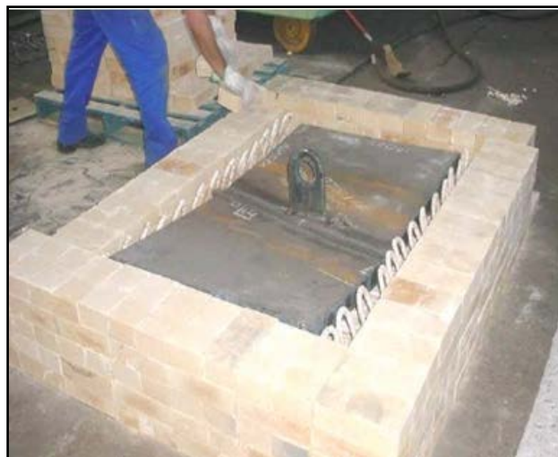
Figure 9. Body-of-proof (BP) under heat treatment.
