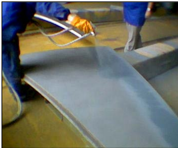
Figure 8. Body-of-proof (BP) painting with spray gun.
