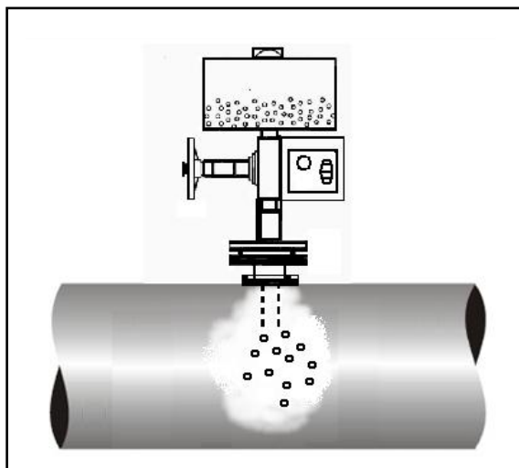
Figure 4. Injection system welded in pipe.
