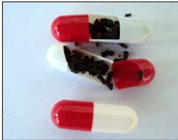
Figure 3. Soluble capsules with solid corrosion inhibitor.
