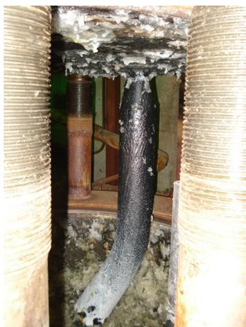
**Figure 2.** The picture of opened HPS with polymeric deposits on the cover and walls.
