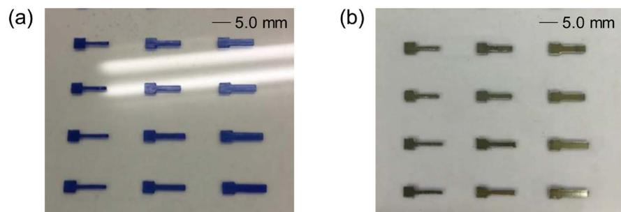
**Figure 2.** Appearance of the pre-structure of the cantilever. (a) Patterned resin prepared by the Step (a) in the **Figure 1**. (b) Nano silver ink-stacked resin prepared by the Step (b) in the **Figure 1**.
