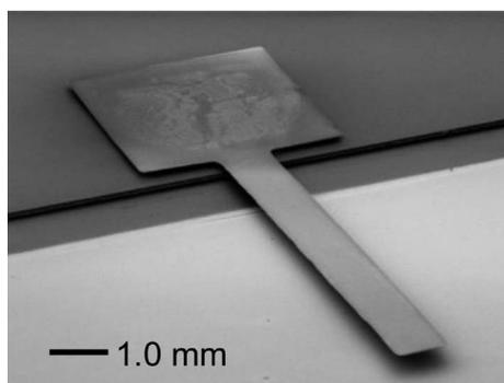
**Figure 3.** SEM image of a fabricated cantilever.
