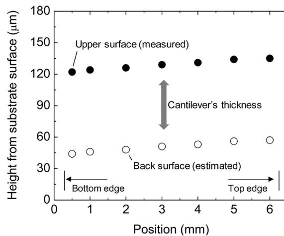
**Figure 4.** Estimated profile of the fabricated cantilever.
