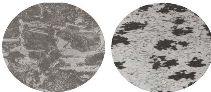
**Figure 4.** Classical effect of heat treatment of white cast iron (left) in affecting microstructural variation leading to the formation of tougher malleable cast iron (right). The hard phases were broken down into their elementary components.
