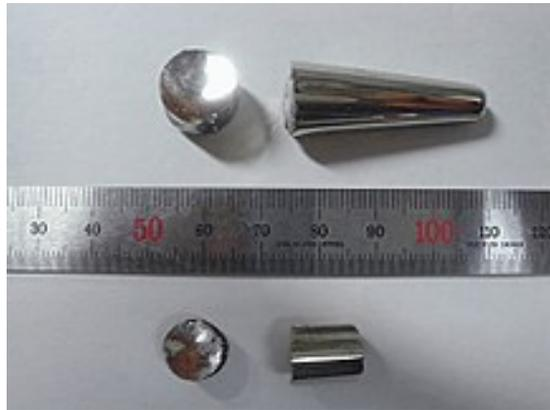
**Figure 7.** Samples of amorphous metal in millimeter length scale [26].
