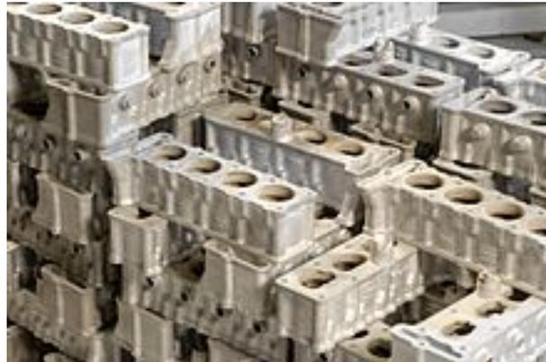
**Figure 6.** Mg alloy motorcycle engine blocks to minimize fuel consumption through weight saving [11].
