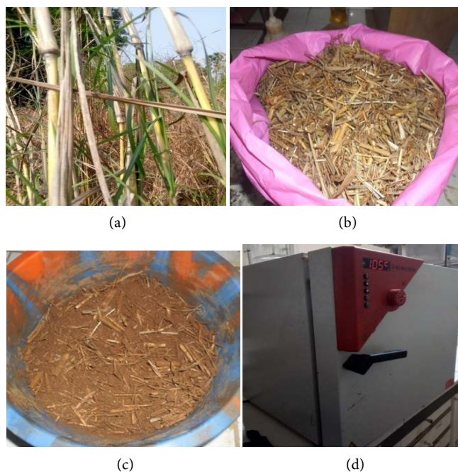
Figure 3. Natural thatch fibres: (a) stem of fibres; (b) dry stem; (c) crushed stem mixed with lateritic soil; (d) oven for drying sample.
