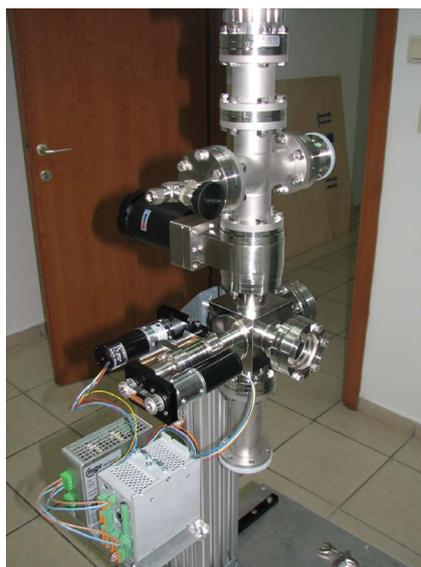
**Figure 3.** Laboratory scale mechanochemical sorption apparatus.
