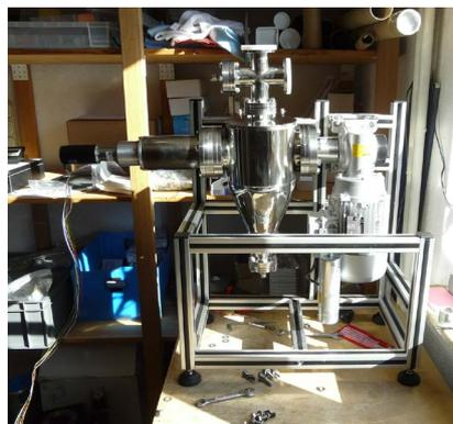
**Figure 4.** Pilot prototype of mechanochemical apparatus.
