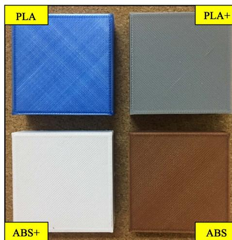
**Figure 4.** FDM 3D printed parts using different filament material.
