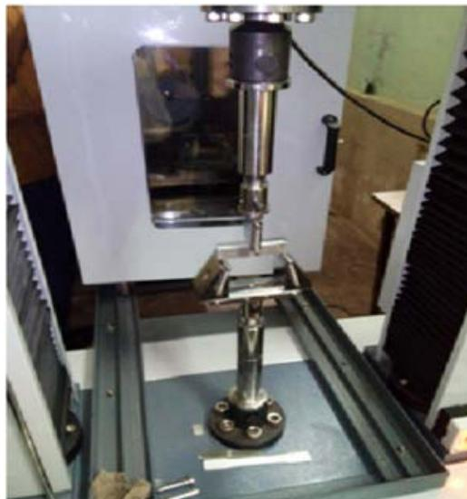
**Figure 1.** Universal testing machine showing the sample position at room temperature.
