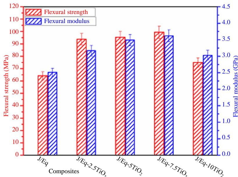
**Figure 4.** Flexural strength and modulus of TiO<sub>2</sub> filled J/Ep composites.
