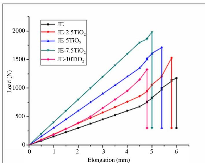
**Figure 1.** Load vs Elongation at break for  $\text{TiO}_2$  filled J/Ep composites.
