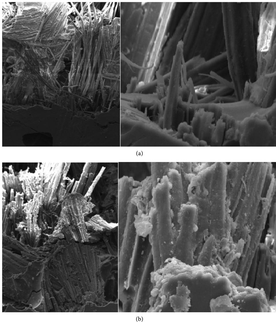
**Figure 5.** Fractographs of tensile failed samples (a) unfilled J/Ep and (b) 7.5 wt% TiO<sub>2</sub> J/Ep composites.
