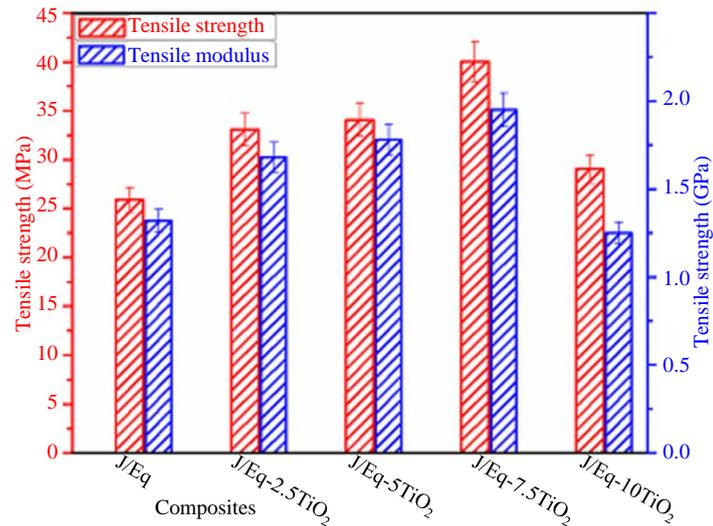
**Figure 2.** Tensile strength and modulus of TiO<sub>2</sub> filled J/Ep composites.
