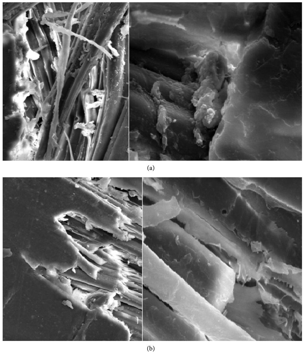
**Figure 6.** (a) Fractograph of bending failed sample of unfilled J/Ep composites; (b) Fractograph of bending failed sample of 7.5 wt% TiO<sub>2</sub> J/Ep composites.
