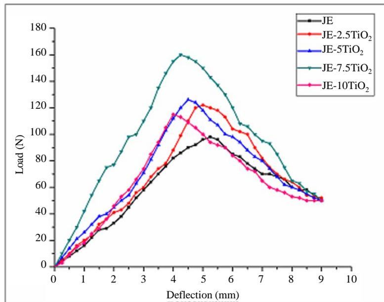
**Figure 3.** Load vs deflection for TiO<sub>2</sub> filled J/Ep composites.
