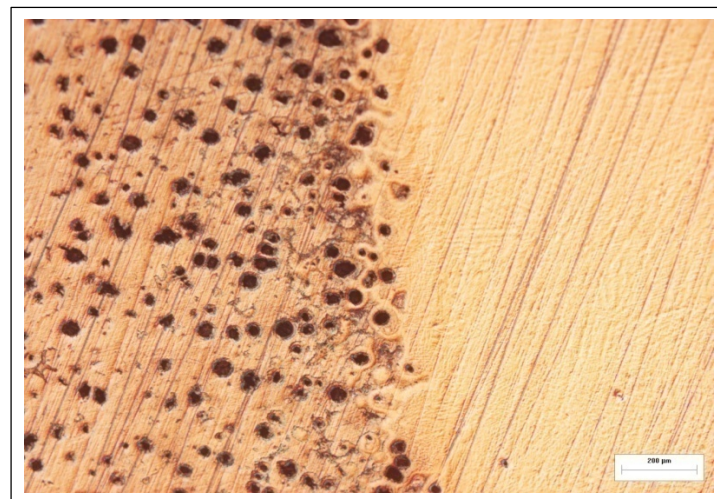
Figure 6. Microstructure of welded 3.35-Si sample (200 X).
