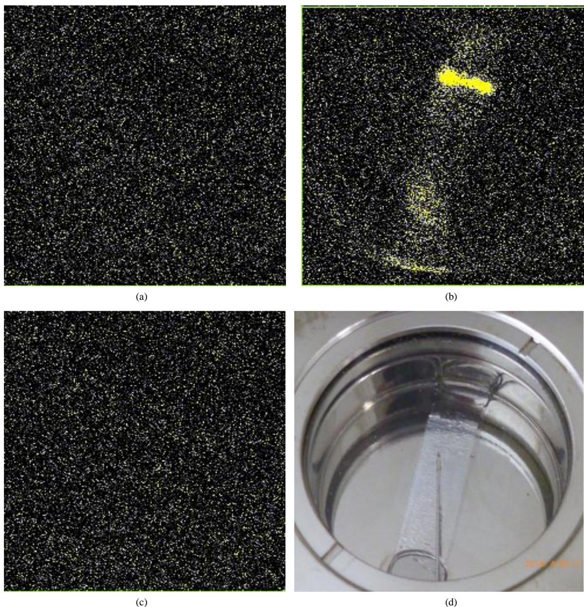
**Figure 3.** Chemiluminescence and after experiment images. (a) Before drip; (b) Immediately after dripping; (c) After drip; (d) After experiment.
