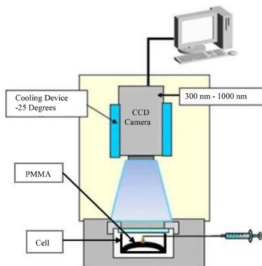
Figure 1. Chemiluminescence image processing device.
