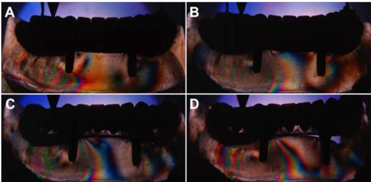
**Figure 3.** Isochromatic fringes in the anterior support areas on the premolar loading.
