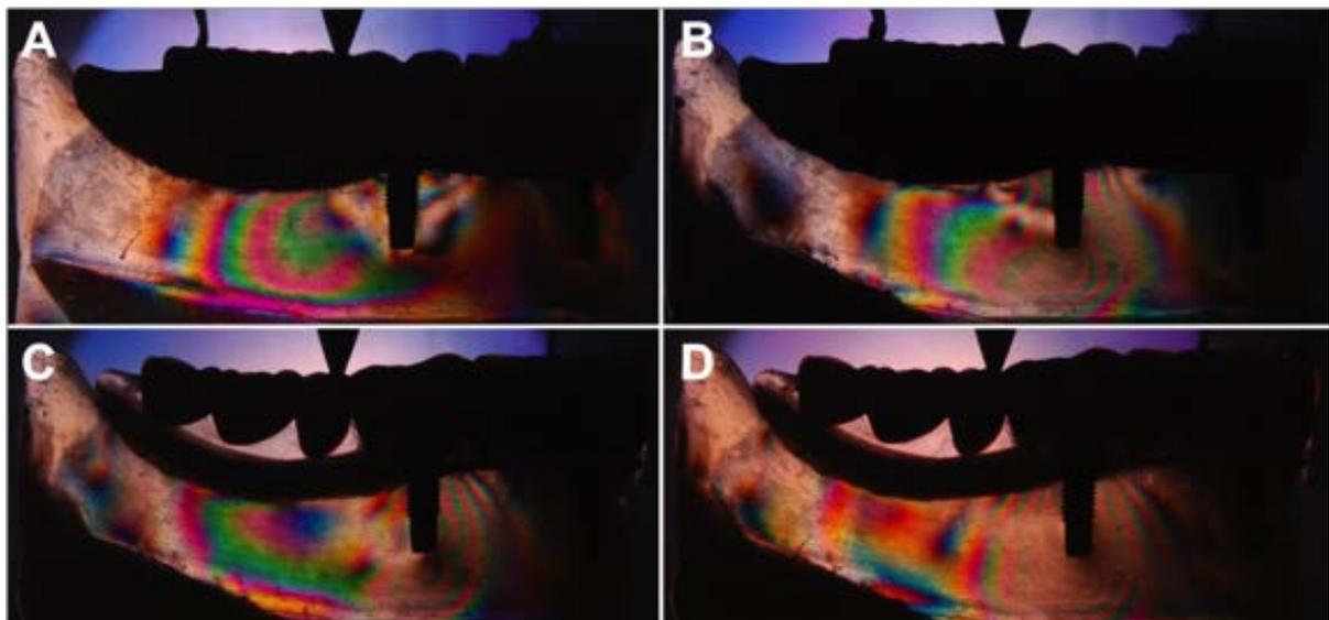
Figure 4. Isochromatic fringes in stress distribution in the anterior/posterior support areas on the premolar loading.
