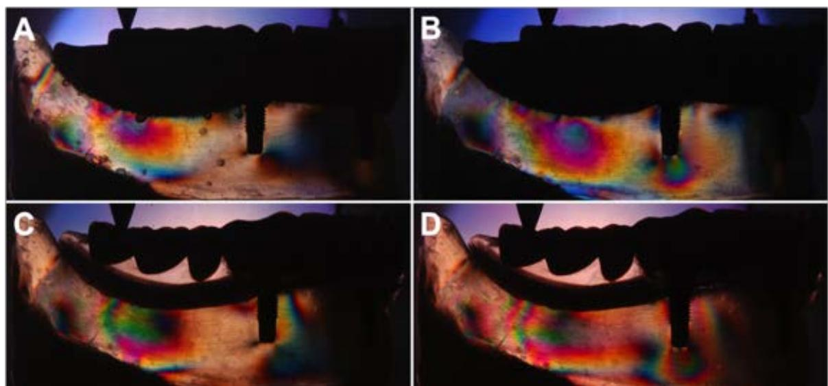
Figure 5. Isochromatic fringes in stress distribution in the anterior/posterior support areas on the molar loading.
