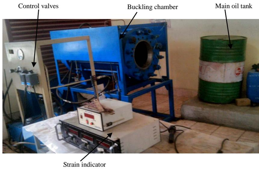
Figure 1. Experimental setup to test buckling due to hydrostatic pressure in FML cylinders.
